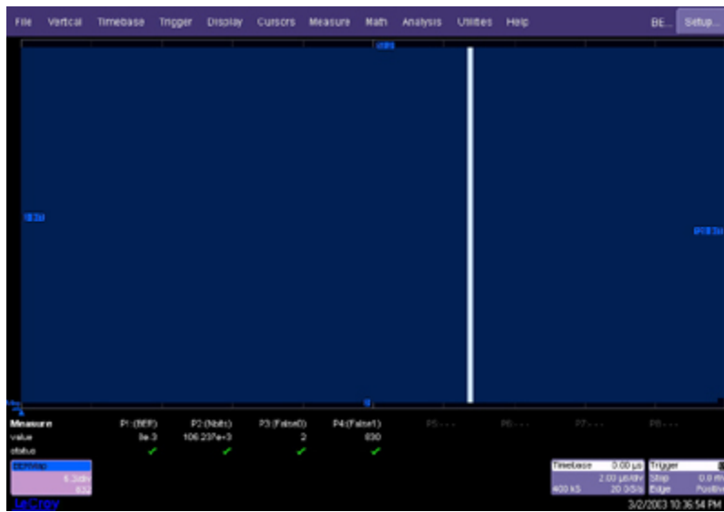
Figure 5-46. Bit Error Map for 127-Bit Pattern Containing Pattern Dependent Errors.
