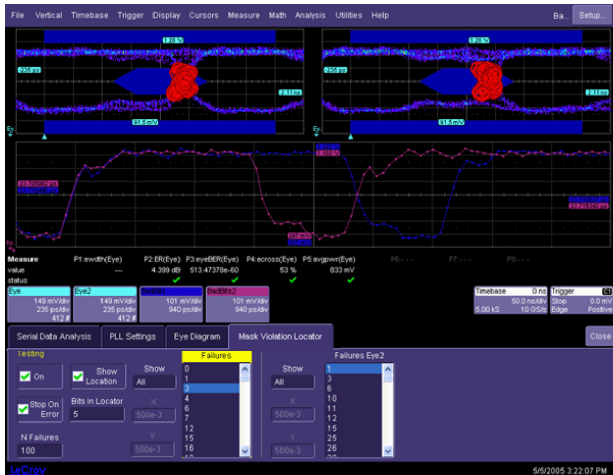
Figure 5-48. Mask Violation Setup.
