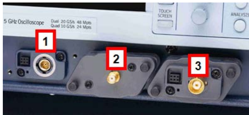
Figure 3-10. BMA Female Connector (1), ProLink BMA-to-SMA Adapter (Installed, 2), and ProLink BMA-to-BNC Adapter (Installed, 3)
