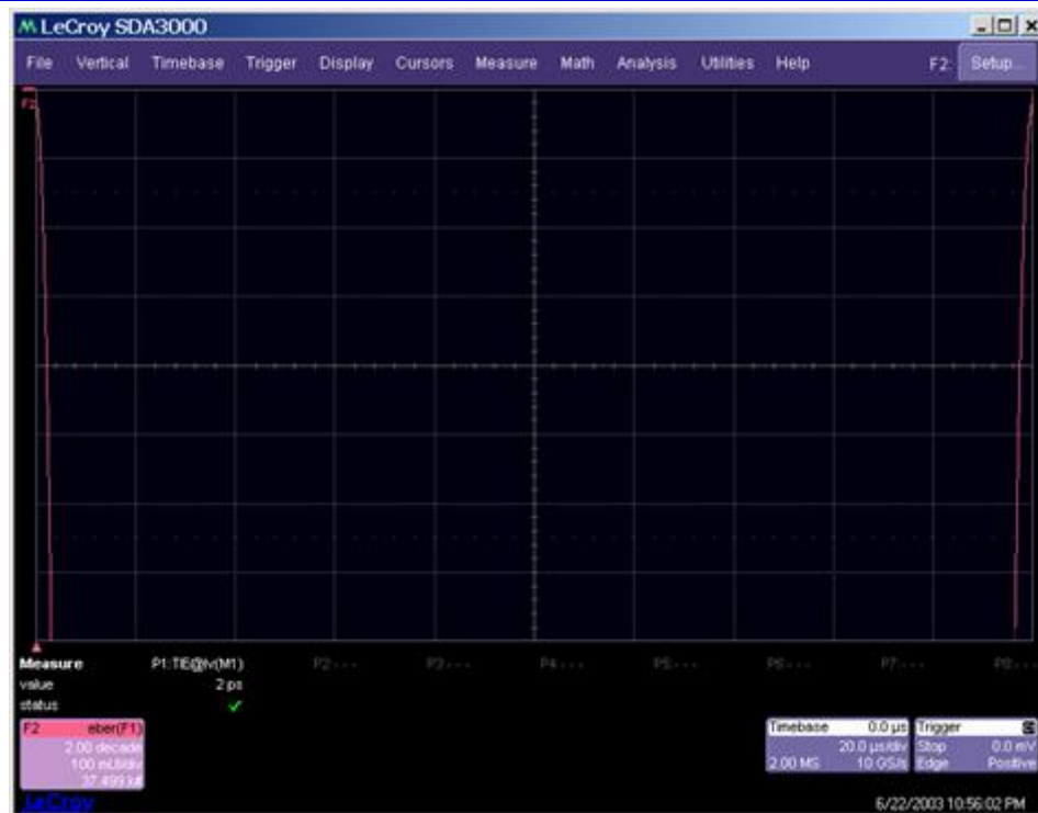
Figure 5-40. The bathtub curve is constructed by rescaling the total jitter curve in Figure 9 to one unit interval, and centering the right side of the total jitter curve at 0 UI and the left side at 1 UI (the left and right sides of the bathtub curve).
