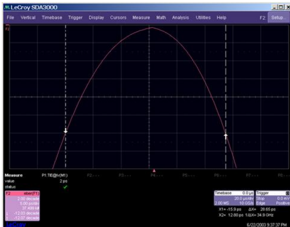
Figure 5-39. Total jitter curve. The vertical values of this curve represent the probability of a data transition occurring at a time represented by the horizontal axis. The horizontal center of the plot is 0 ps. The two markers are placed at the vertical level corresponding to a bit error rate of 10 \text{ e-}12 and the horizontal distance between these two points is the total jitter at this bit error rate.
