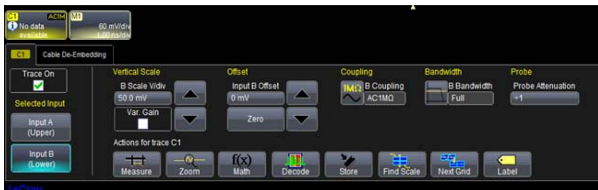
Figure 3-8. The channel screen layout showing Input B's ProBus interface controls setup
