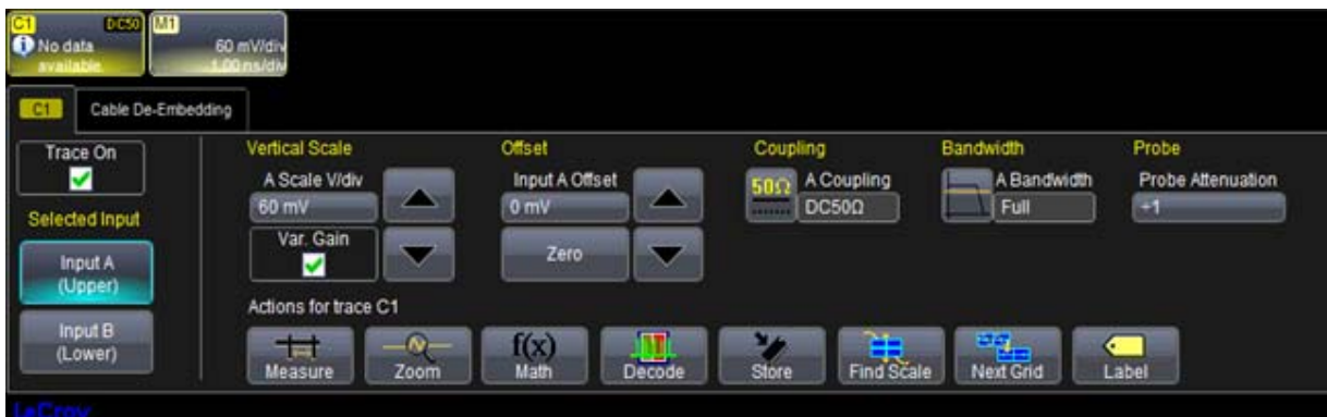
Figure 3-7. The channel screen layout showing Input A's ProLink interface controls setup
